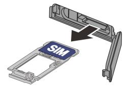
3. Put the tray onto a flat surface and place a microSD card into the tray with the gold contacts facing down as shown below.
