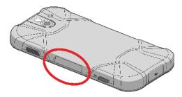
**NOTE:** Make sure the SIM/microSD card slot cover is securely closed to maintain your phone's waterproof seal.
