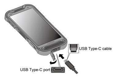
**WARNING:** Only use approved chargers with your device. Incompatible chargers or tampering with the charger port could damage your device and void the warranty.
